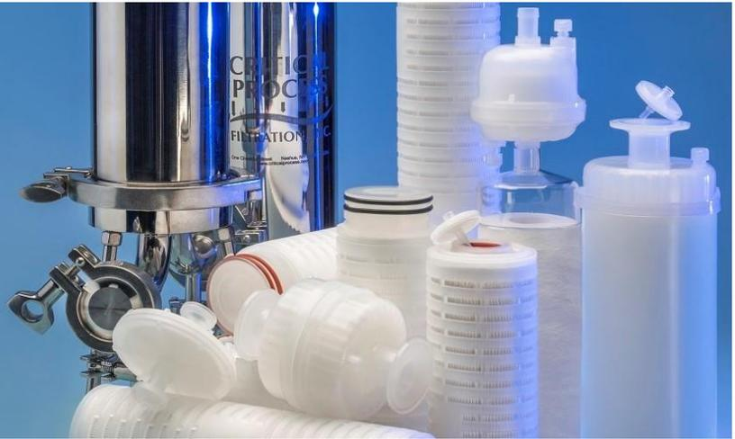
SPS Filters provide a wide selection of validated, single layer Polyethersulfone (PES) cartridge and capsule filters used for the sterilizing of aqueous liquids. Pore sizes range from 0.03 to 1.2  $\mu\text{m}$  and the filter sizes scale from laboratory to full production using identical materials to ensure consistent results.
