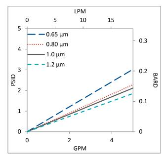
Flow rates for Capsule filters are per square foot of membrane area. The test fluid is water at ambient temperature. Flows are tested using a 2'' capsule filter with  $\frac{1}{2}''$  FNPT inlet and outlet ports. Rates will vary based on end configuration of the capsule.
