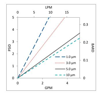
Flow rates for Capsule filters are per square foot of membrane area. The test fluid is water at ambient temperature. Flows are tested using a 2'' capsule filter with 2'' FNPT inlet and outlet ports. Rates will vary based on end configuration of the capsule.
