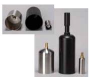
**Gas Blanketing Devices** diffuse the directional energy of the gas flow in tanks and tankers and allow the molecular weight of the gas to blanket gently (laminar flow).
