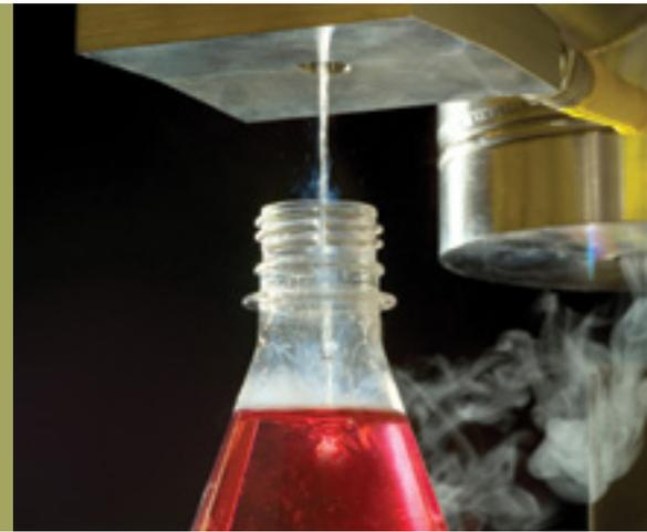
Vacuum Barrier's NITRODOSE® liquid nitrogen injection systems provide the most precise liquid nitrogen dosing to add strength to non-carbonated beverages for light-weight packaging and displace oxygen to extend shelf life.
