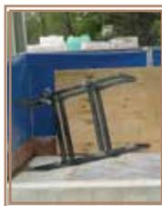
Steel rack buckled, and bent, in addition to causing damage to the cement floor.
