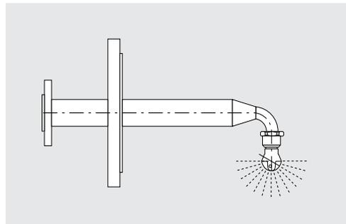
*Bolt-on flanges are also common forms of tank entry. These can be from the top or any other position on the vessel wall, so the length and angle of the inserting pipe can be different in every application.*
