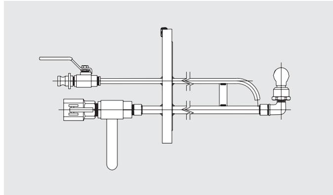
*Sometimes all that is required is a special inlet configuration. This example uses a direct butt-welded connection in a critical reactor mounting.*
