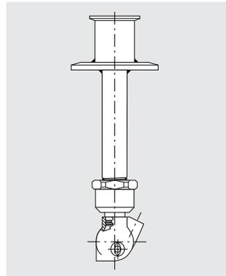
*Applications using tri-clamp nozzle connections and tank spuds are very common in pharmaceutical as well as food and beverage manufacturing. Lechler has produced many variations of this approach.*
