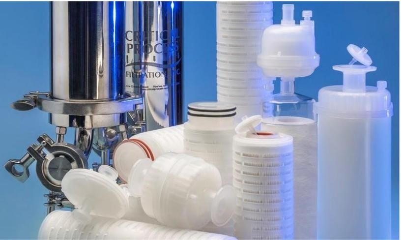
FPD cartridge and capsule filters are constructed with pleated Polypropylene depth media and designed to comply with all FDA requirements for the food industry. FPD filters are used for wine and beer clarification, as well as prefiltering water, food ingredients, cosmetics, chemicals, air and gases. Pore sizes range from 0.10 to 100  $\mu\text{m}$  and filter sizes scale from laboratory to full production using identical materials to ensure consistent results.
