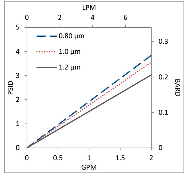
Flow rates for Capsule filters are per square foot of membrane area. The test fluid is water at ambient temperature. Flows are tested using a 2" capsule filter with 1/2" FNPT inlet and outlet ports. Rates will vary based on end configuration of the capsule.
