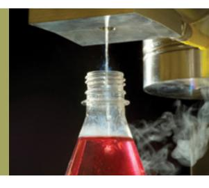
Vacuum Barrier's NITRODOSE® liquid nitrogen injection systems provide the most precise liquid nitrogen dosing to add strength to non-carbonated beverages for light-weight packaging and displace oxygen to extend shelf life.
